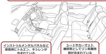
Figure 1 The emission sources of pollutants in a car cabin.
