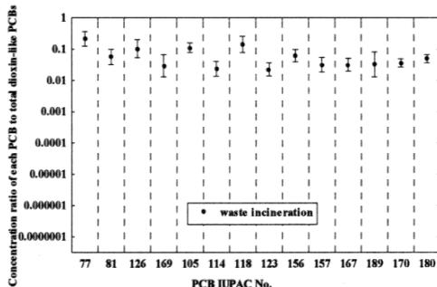
Fig. 2. Ratios of the concentration of each congener to total concentration of dioxin-like PCBs in emissions from 230 waste incinerators<sup>10</sup>. Plots and error bars represent geometric means and geometric standard deviations, respectively.
