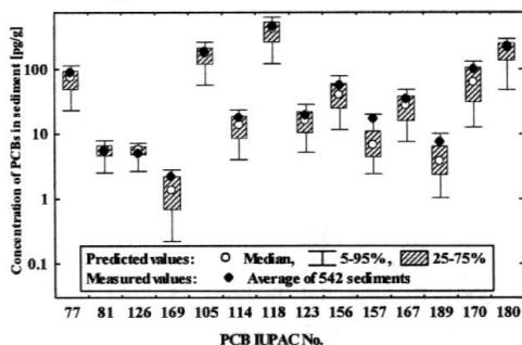
Fig. 4. Comparison of the concentrations of PCB congeners in surface sediments in Japan between measured average values<sup>13</sup> and the values predicted by a CMB approach with a Monte Carlo method. The median and 5th, 25th, 75th, and 95th percentiles of the predicted values in 7,756 iterations are given.
