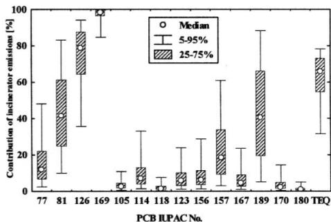
Fig. 5. Contributions of incinerator emissions to the accumulation of PCB congeners in the surface sediments in Japan<sup>13</sup> estimated by a CMB approach with a Monte Carlo method. The median and 5th, 25th, 75th, and 95th percentiles of the predicted values in 7,756 iterations are given.
