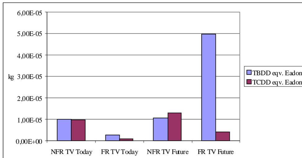
Fig. 5: The emission of TCDD and TBDD equivalents to the air for  $10^6$  TV set over their 10 year life cycle.
