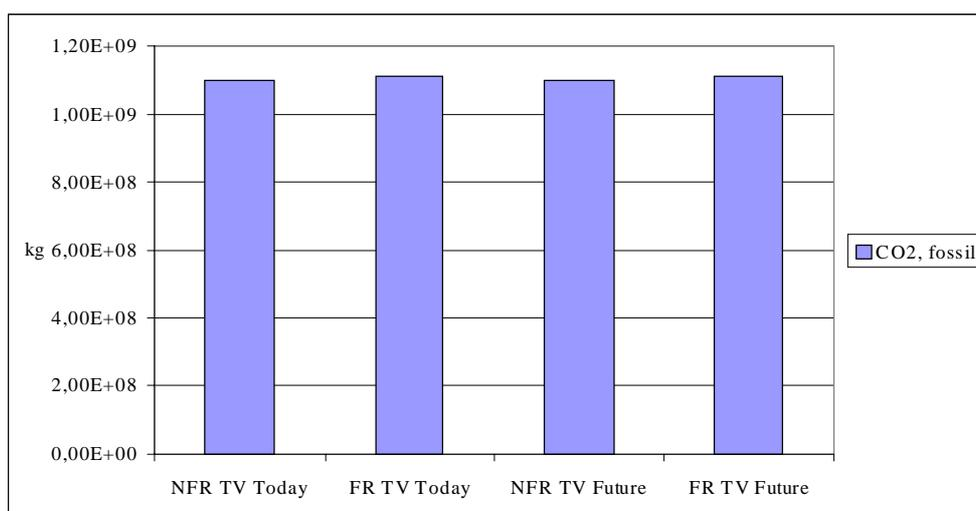
Fig. 3: Comparison of CO<sub>2</sub> emission for 10<sup>6</sup> TV set over their 10 year life cycle.
